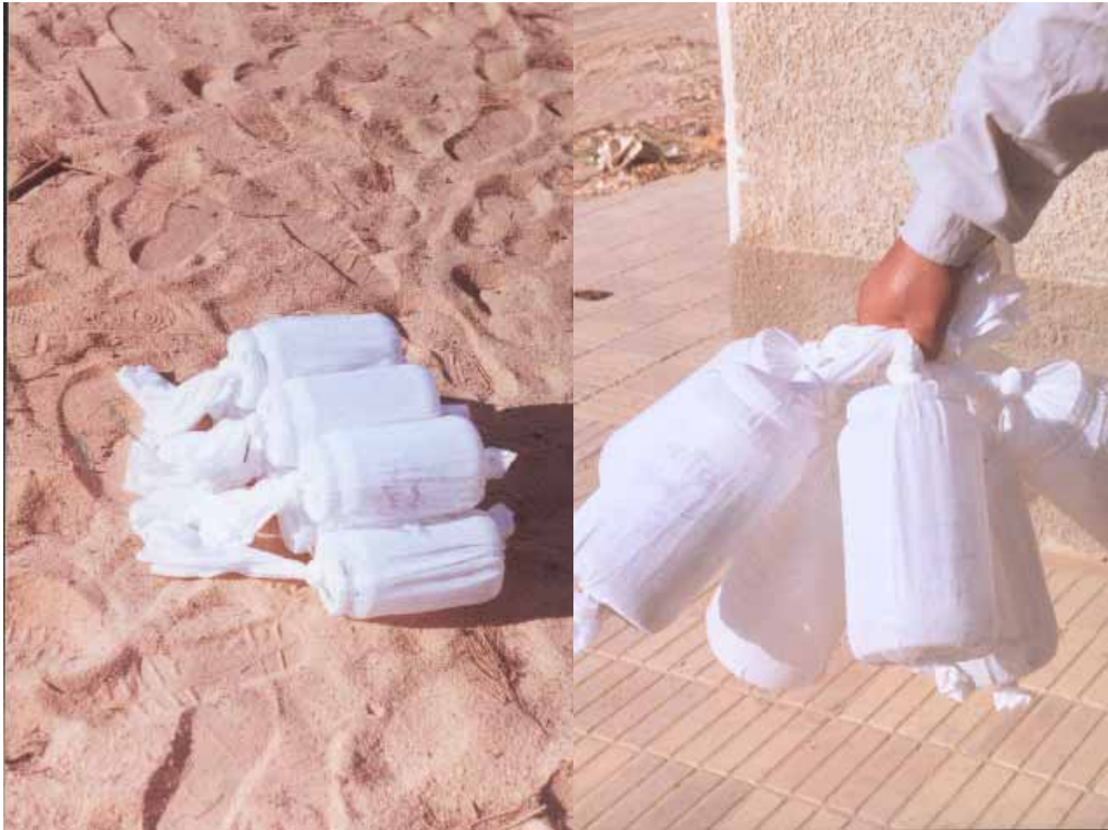
Figure (4) The plastic cage (bottomless plastic jar covered with white long tube of white textile)
